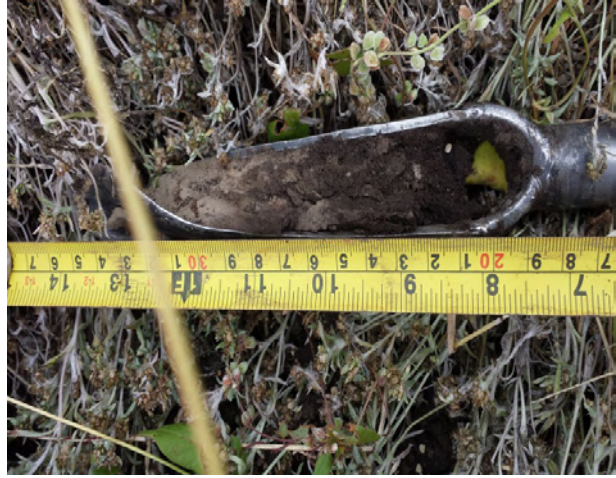
Photo 2: W5 showing mottling within the top 30 cm indicating a temporary type.
