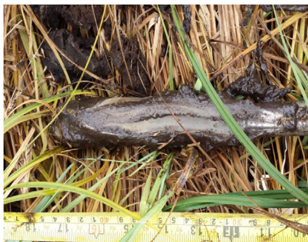
Photo 17: W4 soil characteristics showing wet organic and gleying materials.
